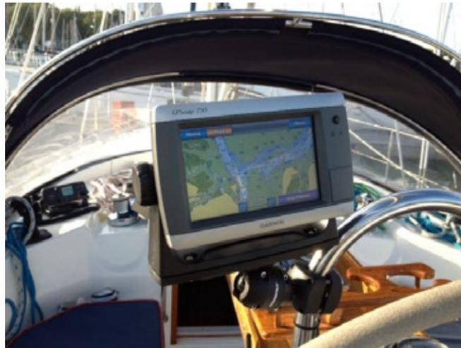
ROKK Adjustable Deck Mount on steering binnacle.
